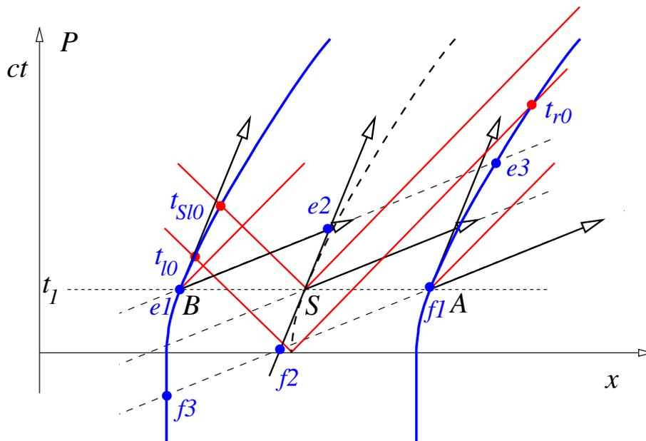
Fig. 4: Dick’s and Jane’s frames  $B$  and  $A$  together with an instantaneously comoving inertial system  $S$ , i.e.,  $S$  does not move along the dashed world line but along a tangent to it.
