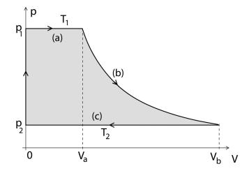
Fig. 3. A pV diagram of the cycle. The process consists of (a) isothermal (and isobaric) expansion, (b) adiabatic expansion, and (c) isothermal compression.
