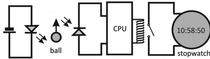
Figure 5. Opto-electronic device for time-interval measuring.
