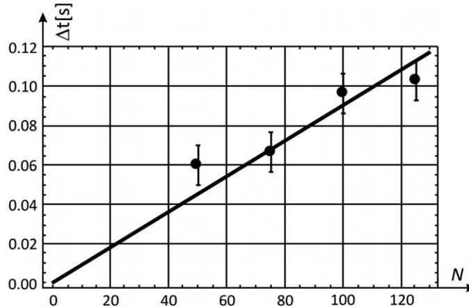
Figure 6. Experimental results: time difference versus number of pendulum turns.
