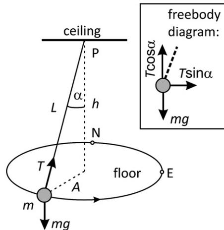
Figure 1. Conical pendulum and corresponding free body diagram.
